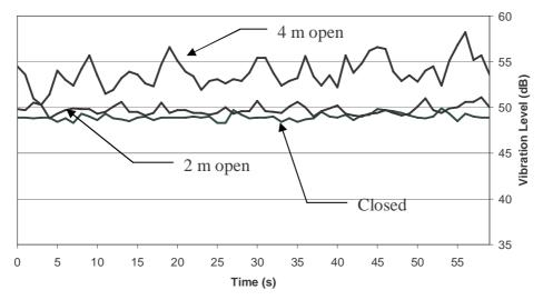
Figure 5: Vibration Survey Wall vibration next to baffle block X-axis (perpendicular to wall)
