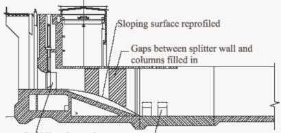
Steel liner in service gate area <sup>1</sup>Baffle blocks reduced in height Figure 2: Modifications to Outlets
