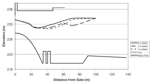
Figure 6: Model Test Results. 75% gate opening and current tailwater level
