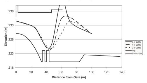
Figure 7: Model Test Results. 75% gate opening and future tailwater level
