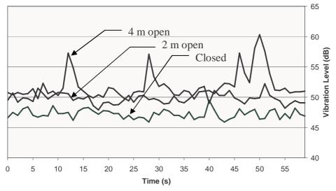
Figure 3: Vibration Survey Gate vibration Y-axis (flow direction)
