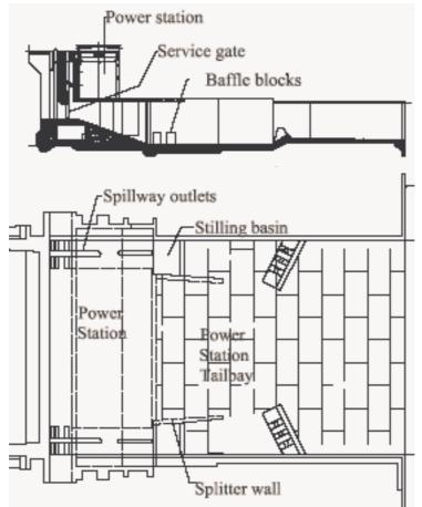
Figure 1: Longitudinal Section and Plan of Outlet Works
