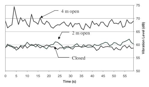
Figure 4: Vibration Survey Slab vibration Z-axis (vertical)
